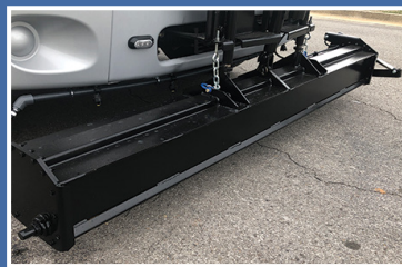
POWERFUL MAGNET TO COLLECT FERROUS MATERIAL
