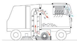
**Dulevo Patented Mechanical-suction-filter system**
