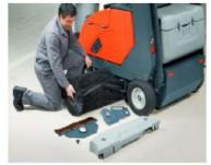
**Convenient Sweeping Cylinders** Tool-free changing of the sweeping cylinder, and protection against wrapping to prevent bearing damage when sweeping up plastic films and straps.
