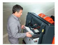
Clean Exhaust Air and Long Operating Times Cassette filter system with a large filter surface and Hako's patented R<sup>2</sup>S filter-cleaning technology.
