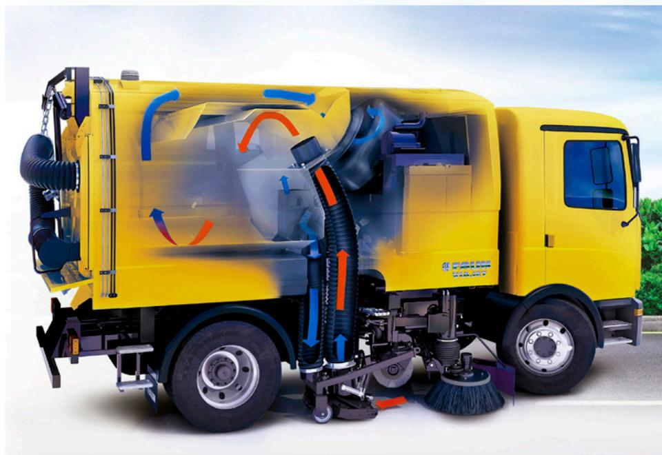
**"Patented Sweeping System"** Our Air Recirculation Technology (**VAST**) allows for sweeping below freezing conditions while expelling 50% less fine dust emission compared to a pure vacuum concept.
