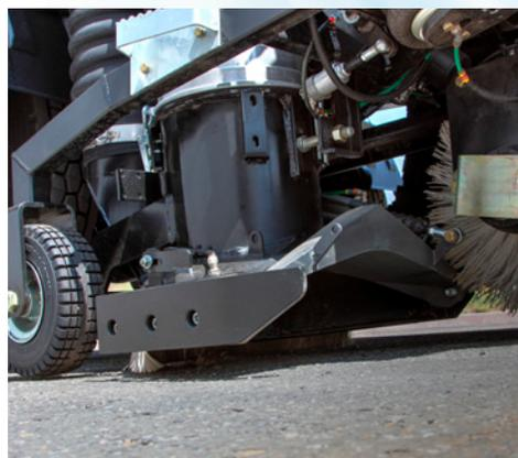
**THE "V-NOZZLE" WILL SWEEP IT ALL** The V-shaped Suction Nozzle with its large aperture, made of 4mm steel, conveys the swept material directly into the suction tube. This design enables the **Global V6AIR** to lift the Heaviest of debris in any application.
