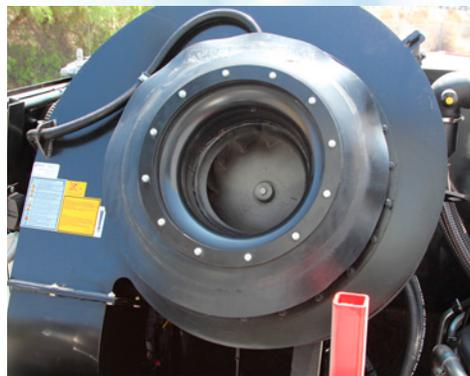
**UNEVEN GROUND, NO PROBLEM** The nozzle is suspended so as to oscillate around its center of gravity, which allows for adjustment to every bump on the sweeping surface. Contact pressure can be easily adjusted, to ensure that every type of surface is swept.
