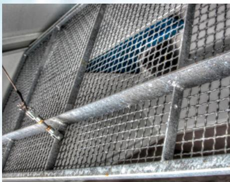
The *Global V6AIR* includes **Galvanized Hopper Screens** that can be easily lowered for cleaning without raising the hopper. The Screening system is designed so that Hopper Screens do not plug up when sweeping light debris such as leaves.
