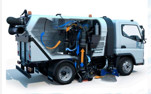
"Patented Sweeping System" Our Air Recirculation Technology (VAST) allows for sweeping below freezing conditions while expelling 50% less fine dust emission compared to a pure vacuum concept.
