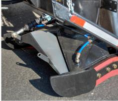
**THE "V-NOZZLE" WILL SWEEP IT ALL** The V-shaped Suction Nozzle with its large aperture, made of 4mm steel, conveys the swept material directly into the suction tube. This design enables the **Global V4AIR** to lift the Heaviest of debris in any application.
