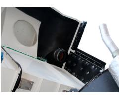
**SILENT PLUS PACKAGE** The "Silent Plus" option utilizes sound supressive material in the engine compartment effectively reducing noise pollution during sweeping to 99 dB(A).
