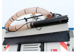
MANUAL SUCTION HOSE The robust rear-mounted suction system provides additoinal vacuum where you need it, such as emptying waste containers, shallow catch basins and loose debris.
