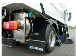
HIGH PRESSURE WASH High Pressure Water Pump, along with hose reel and a lance allow for the ability ot wash sidewalks, containers, etc.
