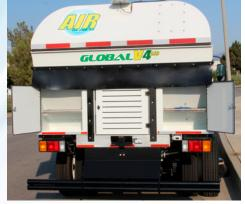
**CONVENIENT STORAGE** The **Global V4AIR** offers two large storage boxes located at the rear of the sweeper.
