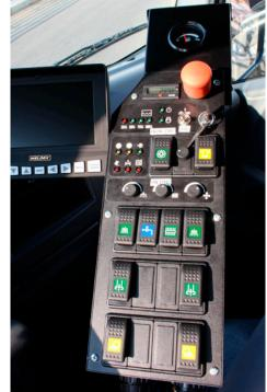
**EVERYTHING AT A GLANCE** The **Global V4AIR** includes central operating panel and easy access to all the functions, while large digital display provides all the necessary information to the operator.
