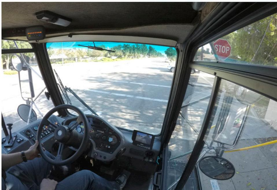
**THE BEST TURNING RADIUS & EXCEPTIONAL VISIBILITY** With the center mounted cab/forward layout the operator has unsurpassed visibility of the road surface as well as pedestrians and surrounding traffic. The 116-inch wheelbase allows for the sweeper to reach a turning radius of 12 1/2 feet, wall-to-wall. With the pickup Head in the center you don't have to worry about what is happening behind you. The **Global R3AIR's** exceptional visibility increases operator and pedestrian safety.
