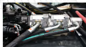
BELOW Elevator Type: optional 11 Flight squeegee with replaceable corded rubber tips; Continuous molded rubber belts combine with optional triple pump option (below) to make Global M4 the logical choice for sweeping heavy debris such as road millings, sand and gravel up to 3-tons per-minute. That is one ton of sand every 20 seconds! Standard leaf gate system assists in picking up large debris, bottles, large branches and leaves.
