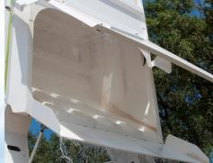
LARGEST HOPPER IN IT'S CLASS Global M4 CNG includes a 5.6 cu/yd hopper capacity compared to 4.5 cu/yd for competitive machines resulting in more curb miles swept between dump cycles. With near Full Useable Capacity, 12,000 Lift Capacity, and the Optional Elevator and Hopper Wash Out System, Global M4 CNG is Affordable, Reliable and Innovative.
