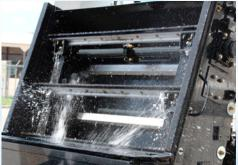
**HEAVY SWEEP PACKAGE** Elevator Type: Standard 11 Flight squeegee with replaceable corded rubber tips; Continuous molded rubber belts combine with standard Heavy Sweep Package make **Global M4 CNG** the logical choice for sweeping heavy debris such as road millings, sand and gravel up to **3-tons per-minute**. That Is one ton of sand every 20 seconds! Standard leaf gate system assists in picking up large debris, bottles, large branches and leaves.
