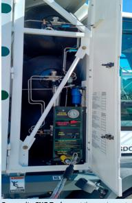
Composite CNG Tanks meet the requirements of ANSI/CS Ar NGV2. USDtOT FMVSS304
