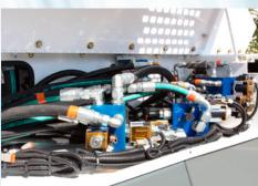
IT'S ALL IN THE OPEN Hydraulic Hoses are NOT hidden in the frame of the sweeper, while all Manifolds and Filters are located in a central location
