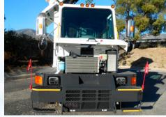
ACCESS IT ALL The Global M4 CNG features many maintenance-friendly attributes, such as a rear swing-out radiator, easy access front mounted AC condenser, brake and windshield washer fluid reservoirs, and cab fresh air filter.
