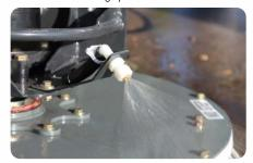
DUST SUPPRESSION SYSTEM • Electric Global M3 includes 230 Gallon Water Tank Capacity combined with Two(2) Diaphragm Water pumps and Two(2) Modes (LOW/HIGH) provide versatility and superb dust control.
