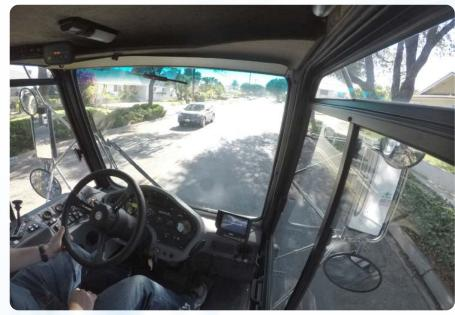
The inherent design of the Electric Global M3 makes it the only choice among 3-wheel mechanical sweepers. With the center mounted/cab forward layout the operator has unsurpassed visibility of the road surface as well as pedestrians and surrounding traffic. The large hopper capacity equals more lane miles swept between dump cycles and the 12.5-foot turning radius makes the Electric Global M3 highly efficient and comfortable.
