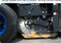
LONG LASTING DIRT SHOES • Polyurethane Dirt Shoes are designed so that operator has sweep over potholes and rail road tracks and will not damage while sweeping. Long Life of 1000 hours is guaranteed. 47" Gutterbrooms assist in cleaning curbs and heavy Road Millings.
