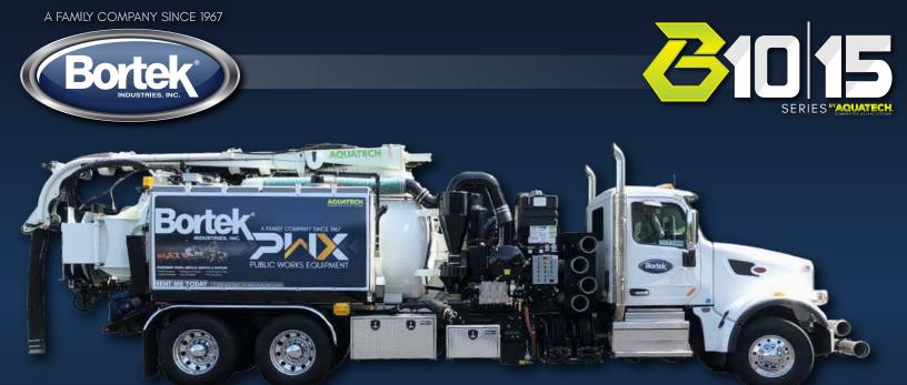
The B10 and B15 Combination Cleaners/Vacuuming Machines are designed to give unsurpassed performance in catch basins, storm sewers, lift stations and treatment plants in municipal and industrial applications.
